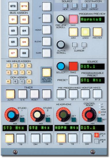
**EVENT COMPUTER** - Virtually all channel switch and knob settings can be named, stored, previewed and recalled in this very user-friendly front panel section (no external computers required). If motorized faders are present their settings are recalled as well.
