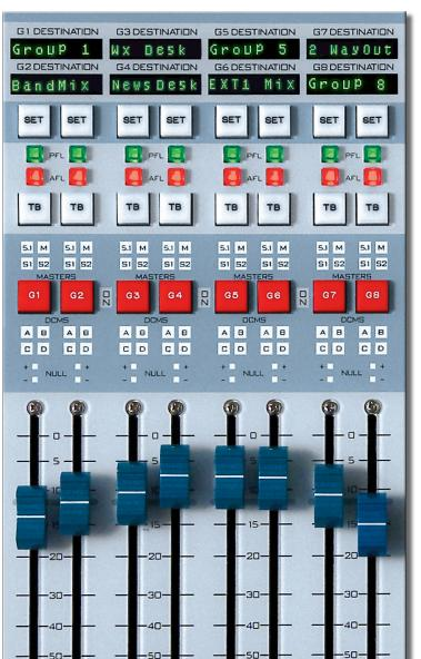
By means of the SET button and the shared resources panel, subgroups may be assigned to any of the four master output faders (5.1, stereo 1, stereo 2, and mono). The bus assign will be indicated by continuous display through the LED backlit windows located above the subgroup master on/off switches.
