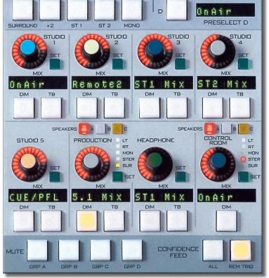
By using the MONITOR SET buttons (left) and the preprogrammed mix switches directly above, these monitors can instantly receive the most frequently accessed mixes. But an extra plus is an array of four programmable monitor source switches above and to the right; even further, access to the entire mix system is possible by means of the upper SELECT encoder and its adiacent TAKE button. With this much monitor power many program segments can be accomplished through this section alone.
