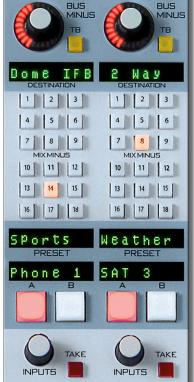
MIX-MINUS (to left) - While input channels all have individual Bus-Minus send controls, the D-5.1 also provides 18 MXM outputs as well to use as a talent foldback system. Assignment is accomplished on the channel's front panel and indicated through LED illuminated switch buttons. This system, combined with the MXM confidence feed system (located on the D-5.1 Dynamic/Confidence Panel) provides a quick convenient foldback function that requires very little operator interaction once set up.
