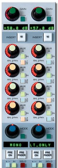
The MXM/AUX master section (to right) provides a consolidated means of setting the master gain level for each of those mixes (gain value indicated in dB). This section also provides talkback to any of these busses and soloing of bus output mixes. PRE/POST buttons allow global settings.
