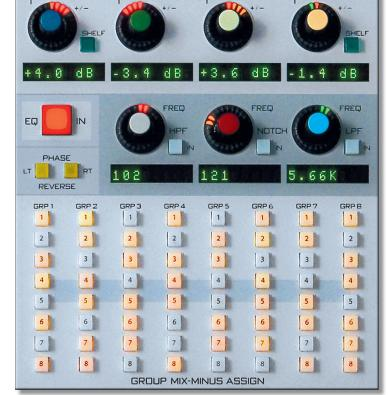
GROUP MIX-MINUS ASSIGN switches allow each of the eight stereo groups access to the first eight of the console's 18 mix-minus busses. This provides a rapid means of developing a mix-minus matrix. The switches are illuminated and positioned directly above the fader panel for clarity of operation.
