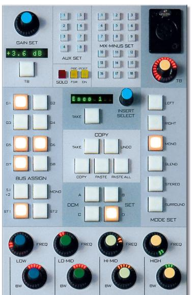
The **COPY/PASTE** section provides a convenient way to duplicate the settings of one input channel strip to any other channel strip, or even to all panel strips—a quick way to initialize a particular operator's setup.
