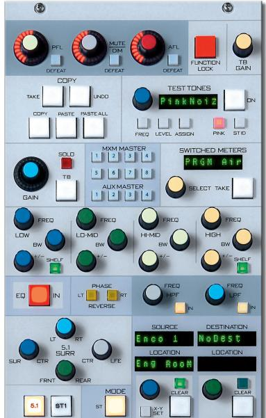
Separate PFL/AFL MASTER level controls (with lightpipe indicators) are provided. DE-FEAT switches can prevent these signals from reaching normal control room monitors if they are being used, for instance, to feed dedicated speakers instead. The MUTE MASTER is used to adjust the level of DIM provided on studio and CR monitor feeds; it can also be defeated.
